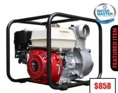
3" Honda® Powered Water Transfer Pump • Honda® GX160 • 3.1 L fuel tank • 3" suction & discharge • 32m max head• 1000 L/min max flow • 27kg MH30-2
